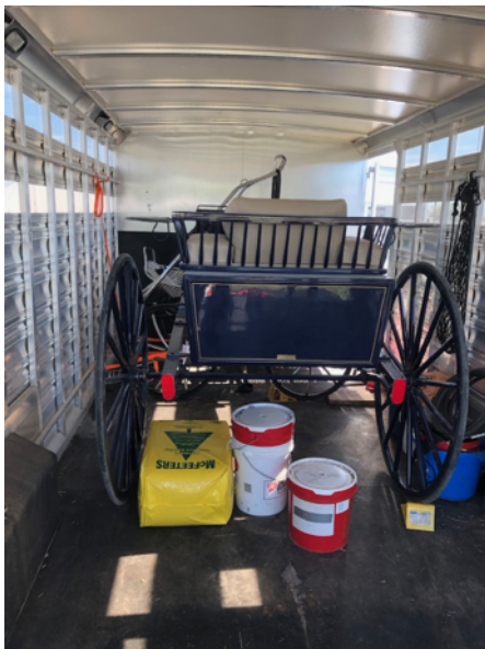
Again, the 8' wide trailer where the marathon vehicle is in front, sideways and secured on the lower rail. The Gig fits easily and the shafts are wrapped, padded and resting on the marathon vehicle. The gate is in the center and the horses can be loaded in the back.
